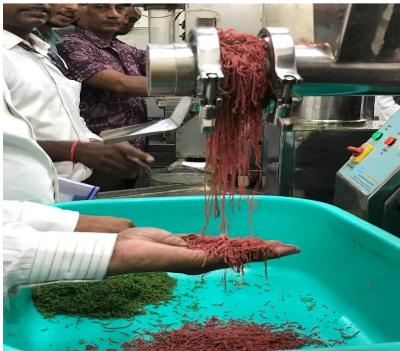
Fig 4: Production of the ornamental fish feed using the single screw extruder and marumerizer
